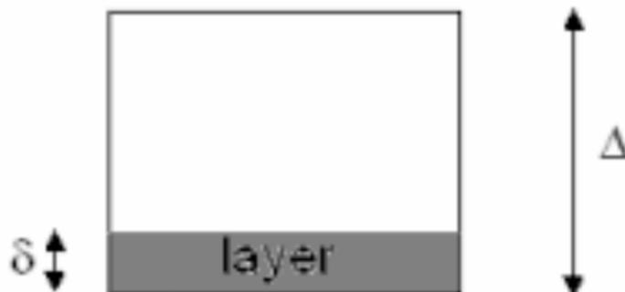
Fig. 2. Scheme of a lower computational cell with a dust deposit in it.
